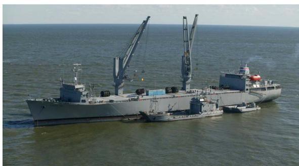
**Figure 1.1:** Cargo Ship Off-Loading Containers Onto Lighter Vessels.
