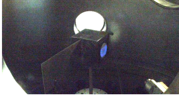
Figure 3.12: Wide Electron Beam for measuring multiple potentials simultaneously
