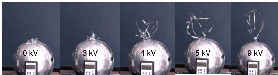
Figure 2: Electrostatic inflation of a gossamer structure
