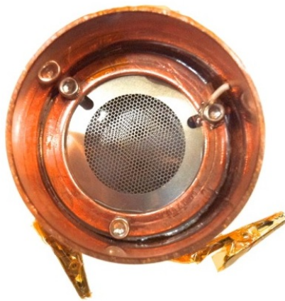
a) Aluminum grid inside test apparatus (view in primary electron velocity direction)
