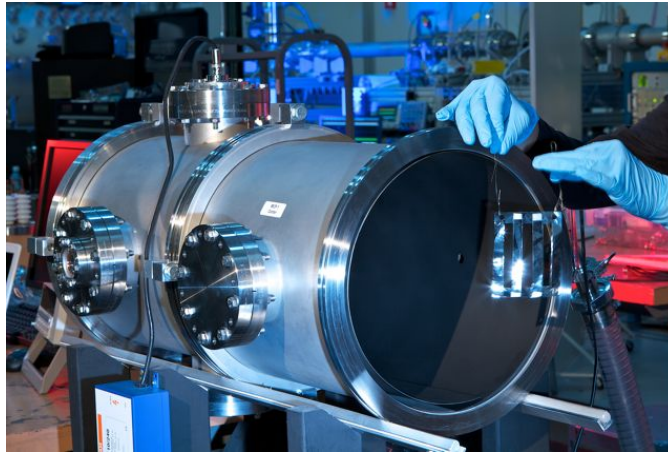
Figure 5: Vacuum chamber used for charging experiments
