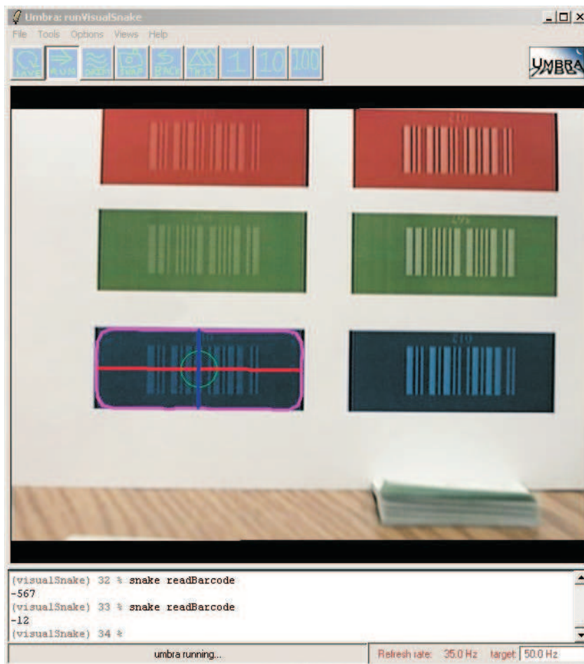
Figure 5. Illustration of an UMBRA module having a snake segment a target region and the barcode routine successfully reading the encoded digits.
