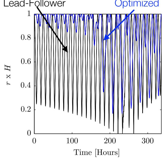
**Particular relative orbits using LROE guidance do improve electrostatic detumble.**
