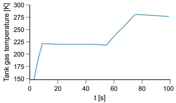
(f) Gas temperature in oxidizer tank
