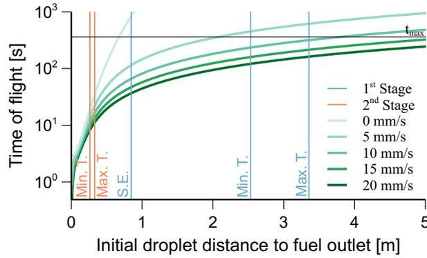
**Figure 13:** Time required by a LOX droplet to reach the bottom of the tank as a function of its initial position and velocity when subject to a  $10^4$  At coil located at the tank outlet. The minimum tank settling length required by the single engine (S.E.), minimum thrust (Min. T.) and maximum thrust (Max. T.) configurations is superposed.
