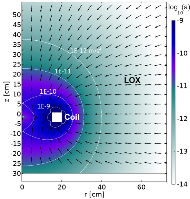
**Figure 5:** Magnetic acceleration contours induced on LOX by a 35 cm diameter coil operating at 1 At.
