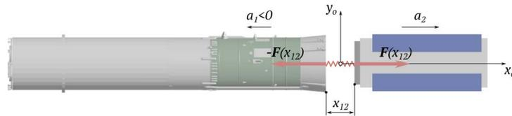
Figure 14: Stage separation model
