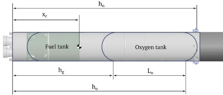
**Figure 1:** Geometrical parameters of a launch vehicle stage.
