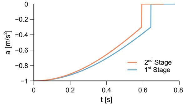
**Figure 2:** Estimated acceleration profile of the 1<sup>st</sup> and 2<sup>nd</sup> stages after separation.
