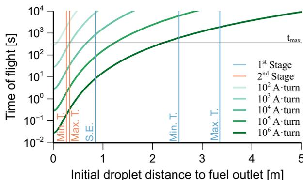
**Figure 6:** Time required by a LOX droplet to reach the bottom of the tank as a function of its distance to the coil and the applied current intensity. The minimum tank settling length required by the single engine (S.E.), minimum thrust (Min. T.) and maximum thrust (Max. T.) configurations is superposed.
