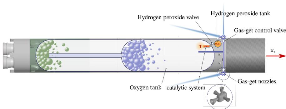
**Figure 9:** Propellant Gasification System
