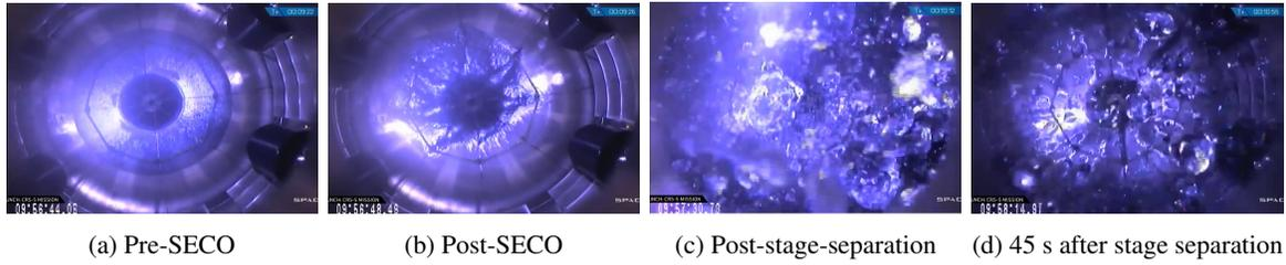
**Figure 3:** Top view of the second-stage LOX tank of SpaceX's Falcon 9 during the CRS-5 mission. Source: [www.youtube.com/watch?v=mVAGoWJuDKk](http://www.youtube.com/watch?v=mVAGoWJuDKk)
