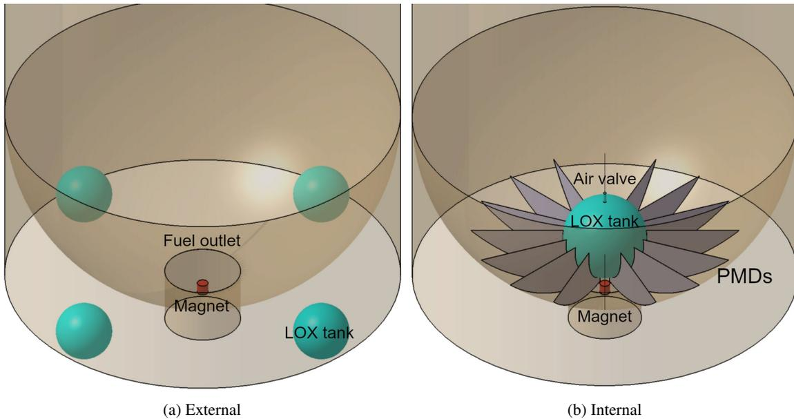
**Figure 8:** Conceptual active liquid retention configurations for Falcon 9's first stage LOX tank.
