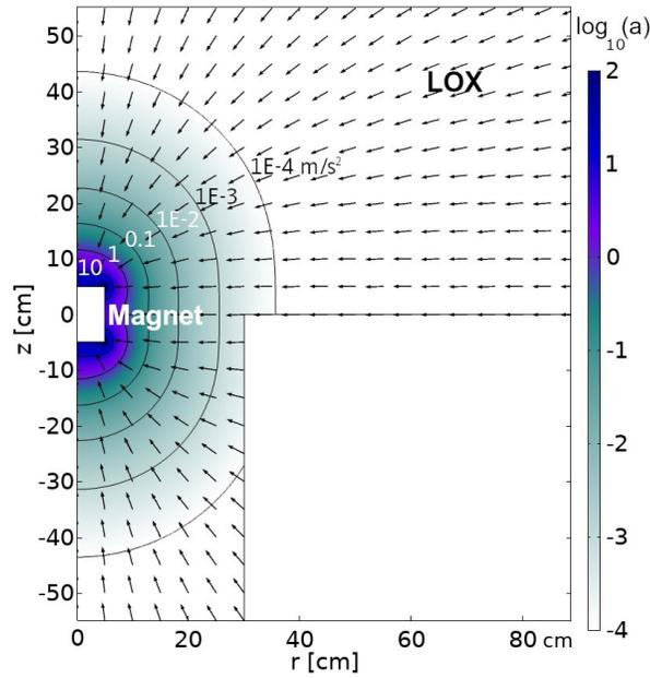
**Figure 7:** Magnetic acceleration field induced by a 5 cm radius 10 cm height praseodymium magnet magnetized at 1300 kA/m.
