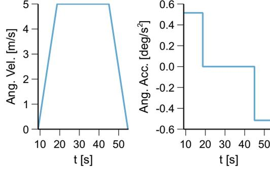
**Figure 11:** Angular velocity and angular acceleration profiles of the 1<sup>st</sup> stage during flip around maneuver using the attitude control nozzles with a total thrust of 1 kN
