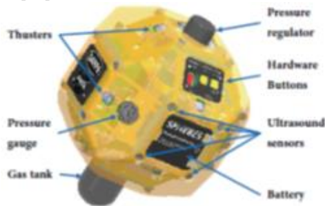
Figure 1: Main components (left) and basic properties (right) of a SPHERE Satellite [18, 19]
