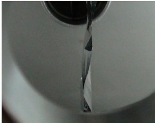
**Figure 3.5:** *Inflation experiment with ribbed structure (Configuration B) at 5kV being performed in the vacuum chamber*
