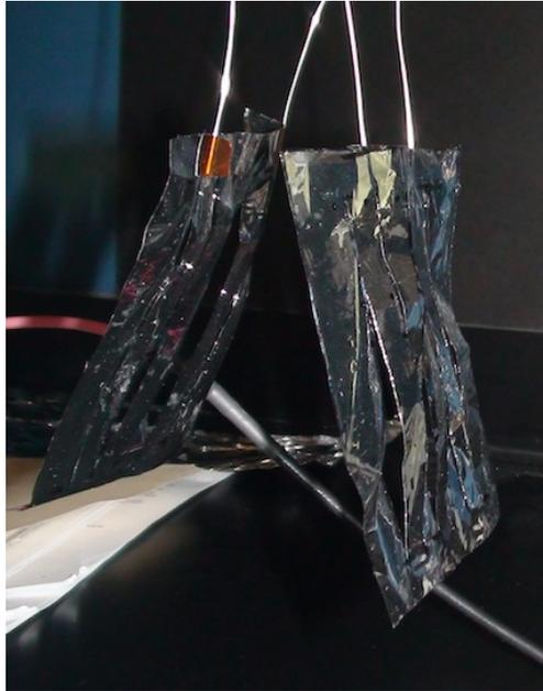
**Figure 3.2:** *Atmospheric inflation experiment with slitted membrane sheet at 10 kV*
