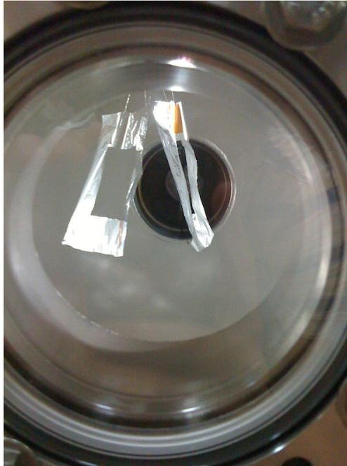
**Figure 3.4:** *Inflation experiment with membranes at 5kV (configuration A) being performed in the vacuum chamber*
