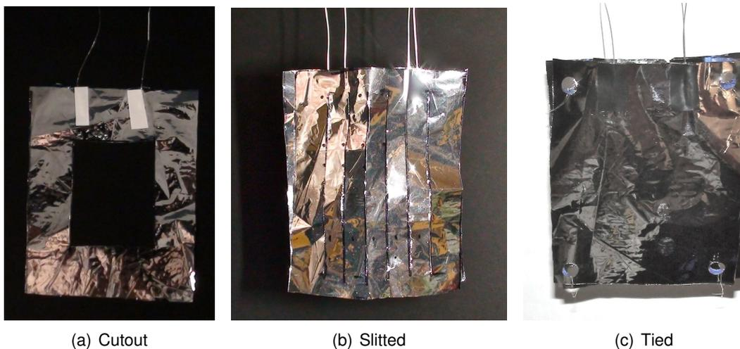
**Figure 3.3:** Photos of several membrane structures tested in atmospheric and vacuum conditions
