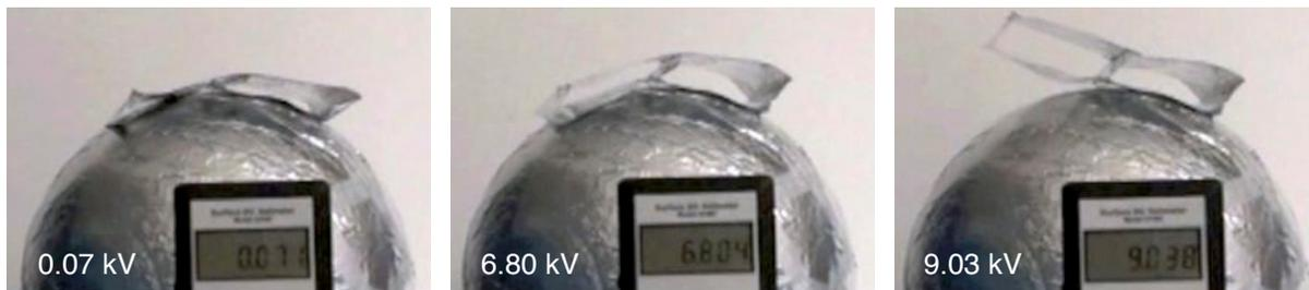
**Figure 1.4:** *Atmospheric Electrostatic Inflation Experiment of a Box-Like Membrane Structure*
