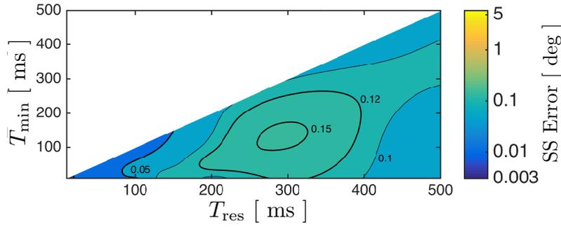
(c) Static bias sweep for the CEIL pulse rounding method.
