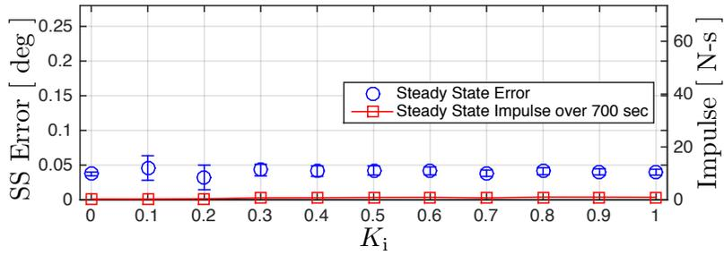
(b)  $K_i$  sweep using the ROUND pulse rounding method.
