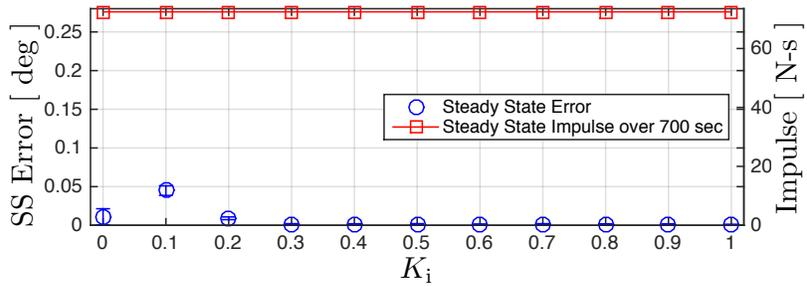
(c)  $K_i$  sweep using the CEIL pulse rounding method.
