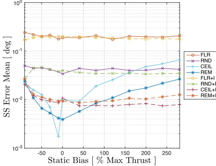
**Figure 3:** Static bias sweep showing results for all methods. Dashed lines indicate use of an integral term.
