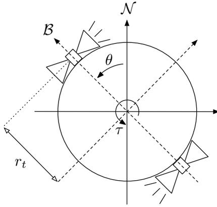
**Figure 1:** A simplified spacecraft with thrusters.
