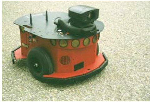
Figure 3: ActivMedia Robotics Pioneer 3-DX robotic vehicle with digital camera system
