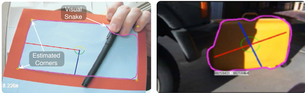
a) Visual Snake Tracking a Partially Obscured Square Target and Estimating the Corner Locations 24 b) Visual Snake Tracking a Yellow Suit-Case Outdoors with Severe Lighting Variations 15
