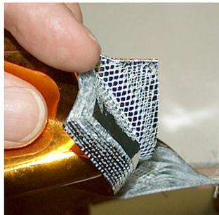
**Figure 2.23:** *Multi Layer Insulation with non-conducting mesh shown*
