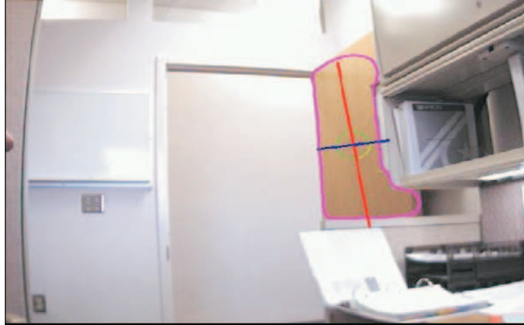
Figure 1. Statistical Pressure Snake Tracking the Wood Door
