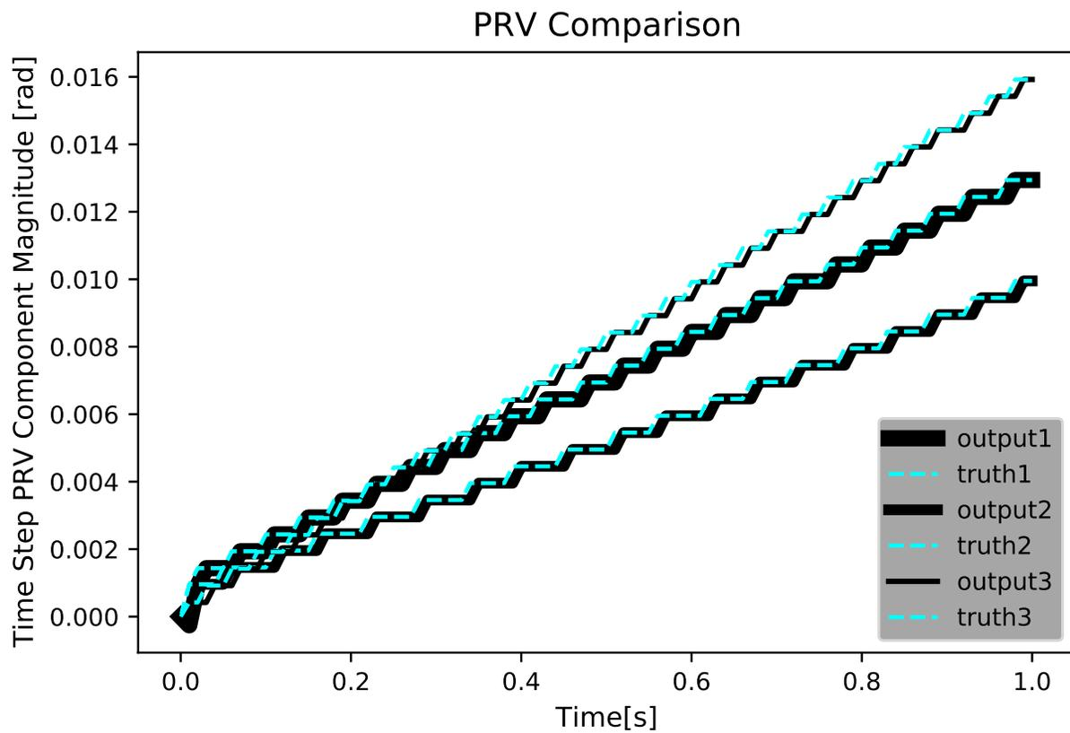
**Fig. 20:** Plot Comparing Time Step PRV Truth and Output for test: discretization. Note that 1, 2, and 3 indicate the components of the principal rotation vector.
