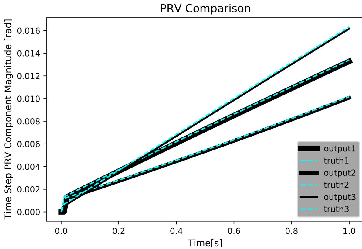
**Fig. 4:** Plot Comparing Time Step PRV Truth and Output for test: clean. Note that 1, 2, and 3 indicate the components of the principal rotation vector.
