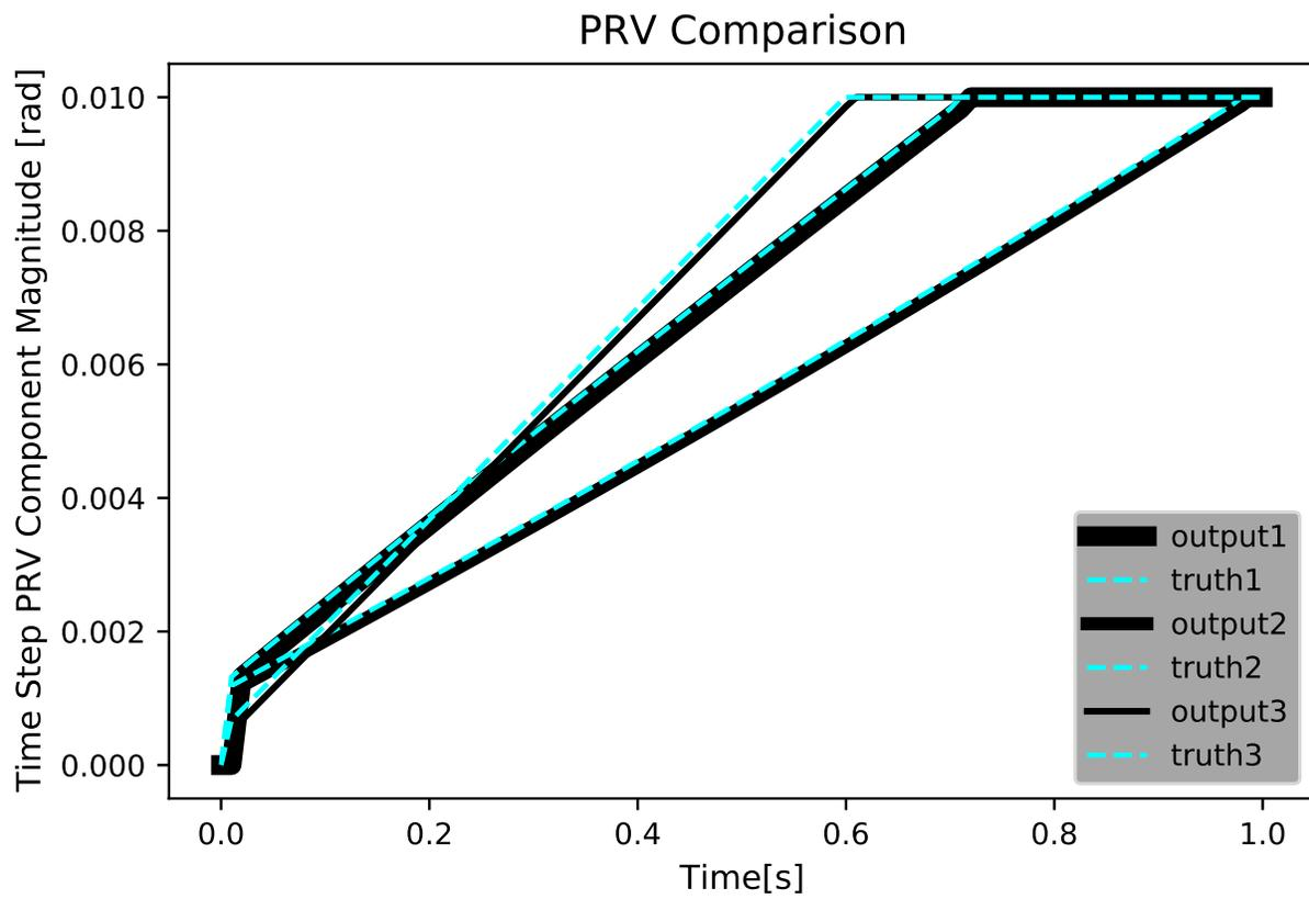
**Fig. 16:** Plot Comparing Time Step PRV Truth and Output for test: saturation. Note that 1, 2, and 3 indicate the components of the principal rotation vector.
