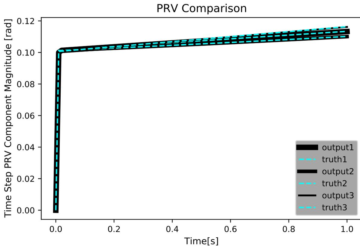
**Fig. 12:** Plot Comparing Time Step PRV Truth and Output for test: bias. Note that 1, 2, and 3 indicate the components of the principal rotation vector.
