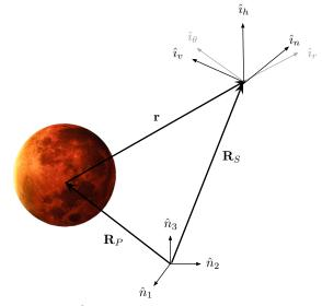
**Fig. 2:** Illustration of the inertial frame  $\mathcal{N} : \{\hat{n}_1, \hat{n}_2, \hat{n}_3\}$  and the orbit frames Hill  $\mathcal{H} : \{\hat{i}_r, \hat{i}_\theta, \hat{i}_h\}$  and Velocity  $\mathcal{V} : \{\hat{i}_n, \hat{i}_v, \hat{i}_h\}$ .
