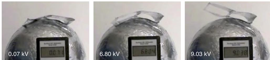
Fig. 5. Electrostatic inflation of a test sandwich structure, from 0 kV to 9 kV.
