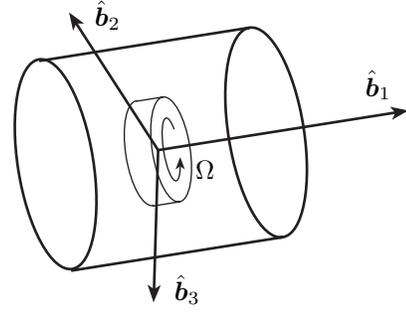
Figure 6: Illustration of a dual-spin spacecraft with the wheel rotation axis aligned with a spacecraft principal axis.
