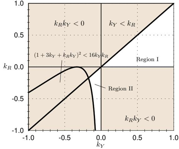
Figure 8: Linearized Gravity Gradient Spacecraft Stability Regions
