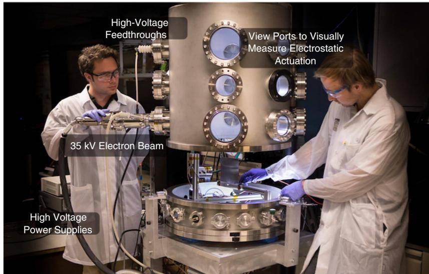
Fig. 1 ECLIPS space environment simulation testbed.
