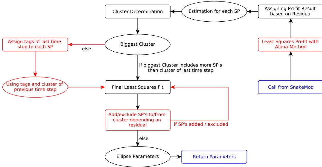
Figure 4.2.: Flowchart of the ellipse identification algorithm with modified parts in red.
