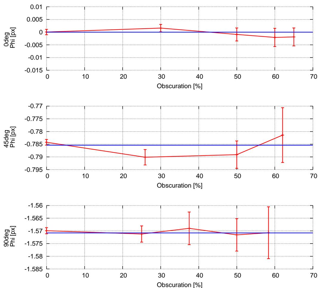
Figure 4.10.: Mean  $\mu_\varphi$  and standard deviation  $\sigma_\varphi$  of  $\varphi$  depending on grade of obscuration.
