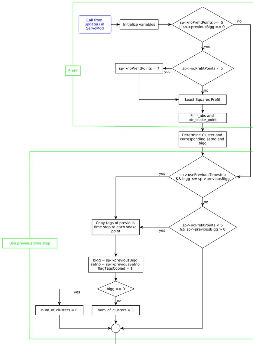
Figure A.1.: Detailed Flowchart of Ellipse Identification Algorithm - Part 1
