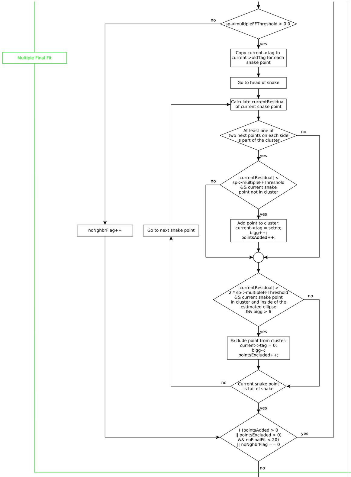
Figure A.3.: Detailed Flowchart of Ellipse Identification Algorithm - Part 3
