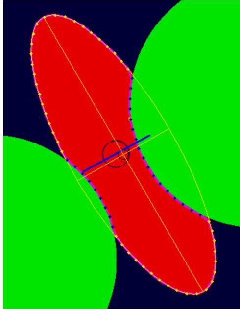
Figure 4.18.: Identification of ellipse with segmented contour.
