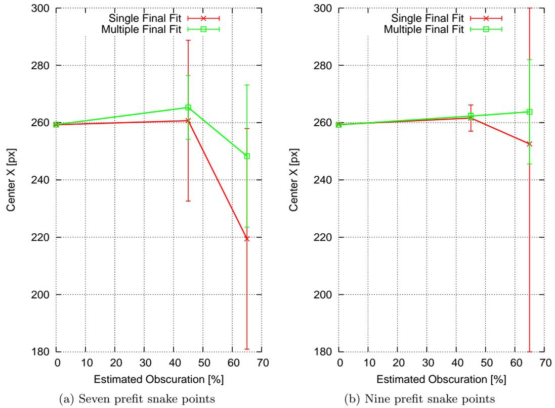
Figure 4.16.: Mean and standard deviation of  $x_c$  using seven or nine profit snake points.
