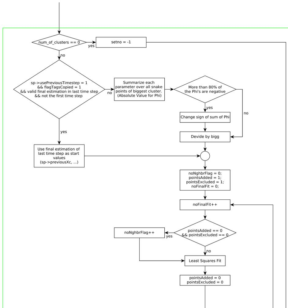
Figure A.2.: Detailed Flowchart of Ellipse Identification Algorithm - Part 2
