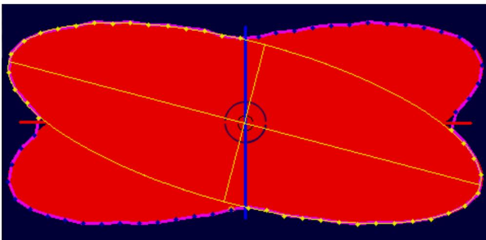
Figure 4.5.: Two ellipses differing only in  $\varphi$  as test case for  $w_\varphi$  with  $\Delta\varphi = 30^\circ$ .
