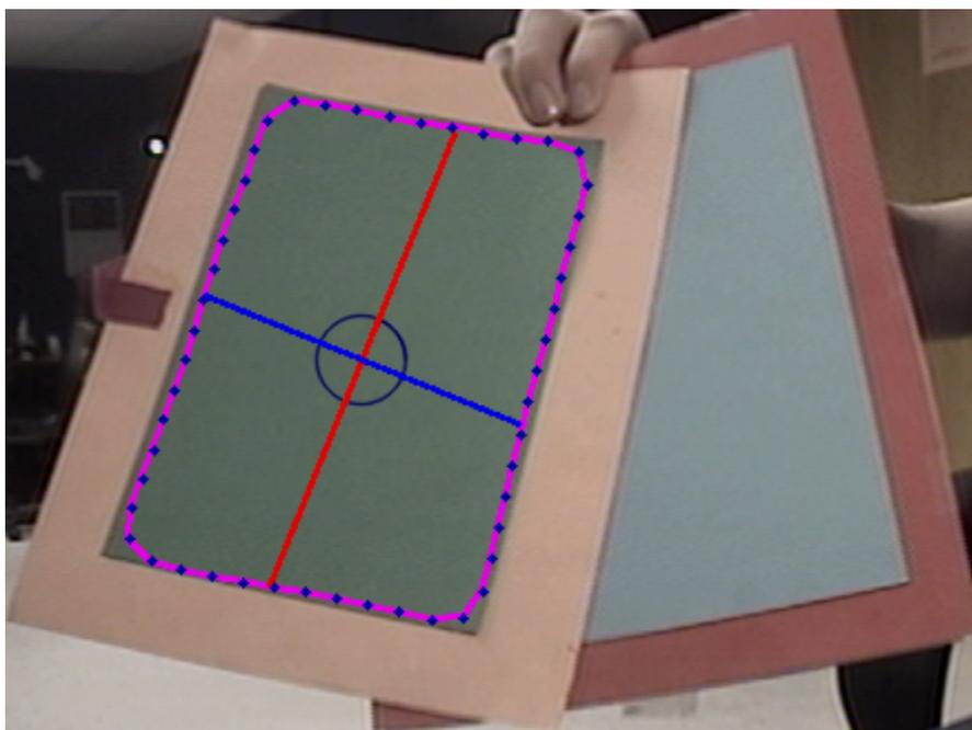
Figure 2.1.: Statistical pressure snake in violet with blue snake points defining the spline. The red and blue lines show the calculated principle axes of the object.
