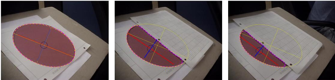
Figure 4.15.: Three different grades of obscuration for real image comparison of single and multiple final fit.
