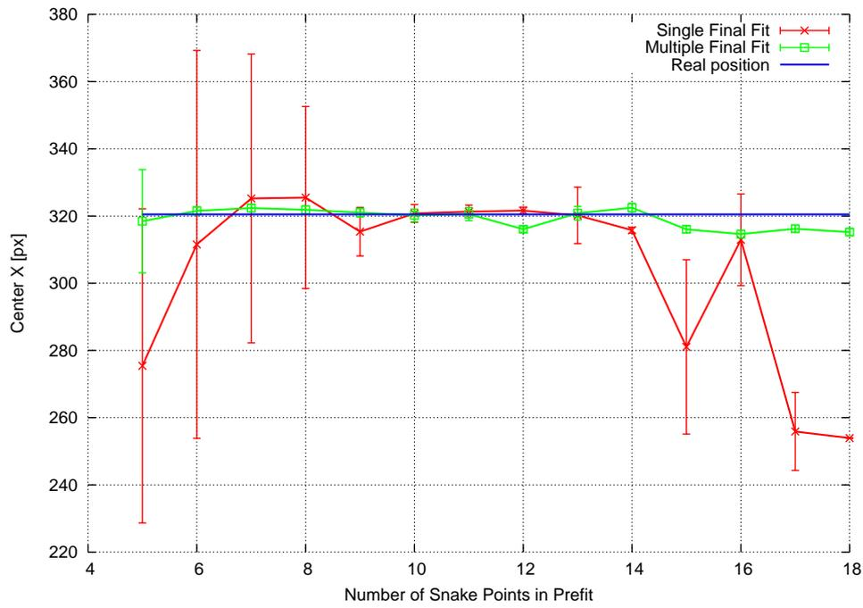
Figure 4.12.: Accuracy of the estimation for  $x_c$  using single and multiple final fit.
