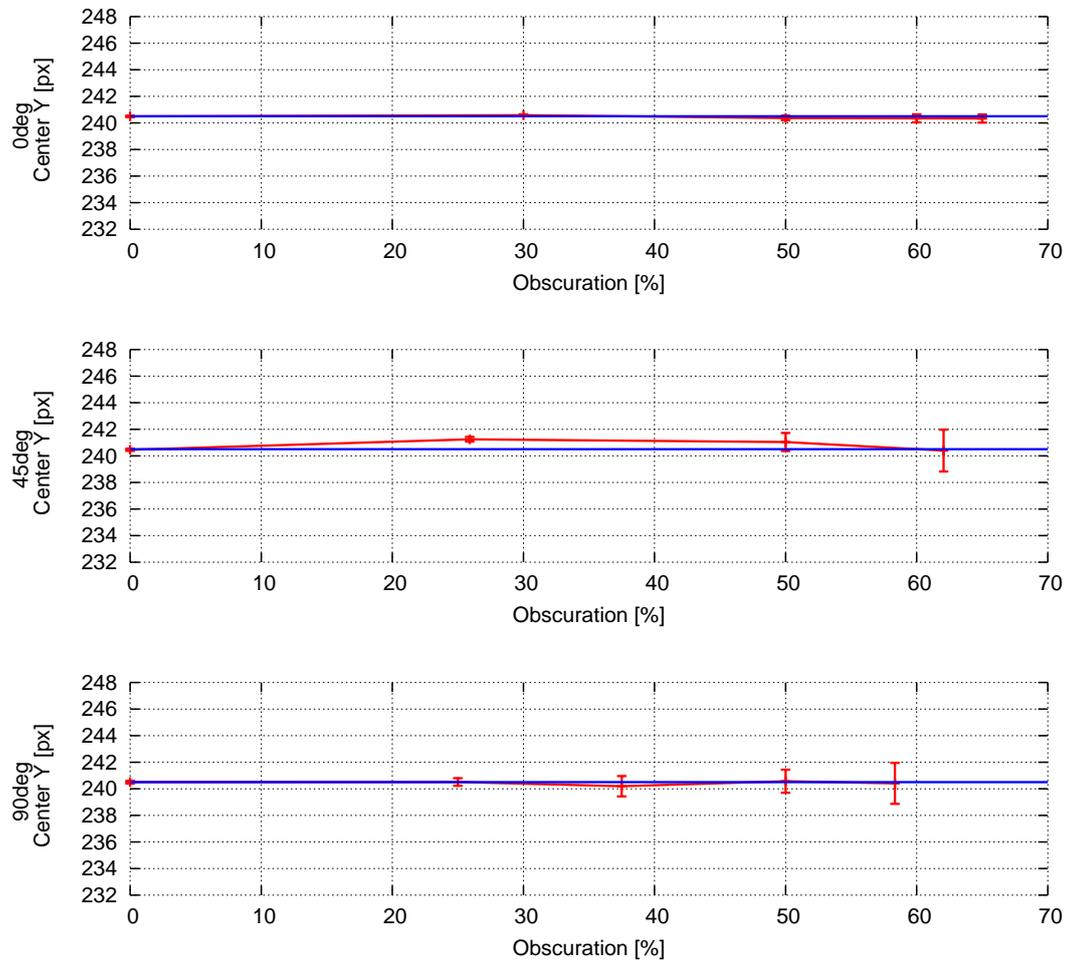
Figure 4.9.: Mean  $\mu_{y_c}$  and standard deviation  $\sigma_{y_c}$  of  $y_c$  depending on grade of obscuration.
