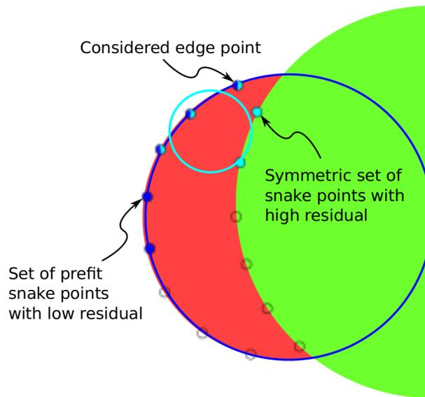
Figure 3.5.: Two different sets of prefit snake points, one with high and the other one with low residual.
