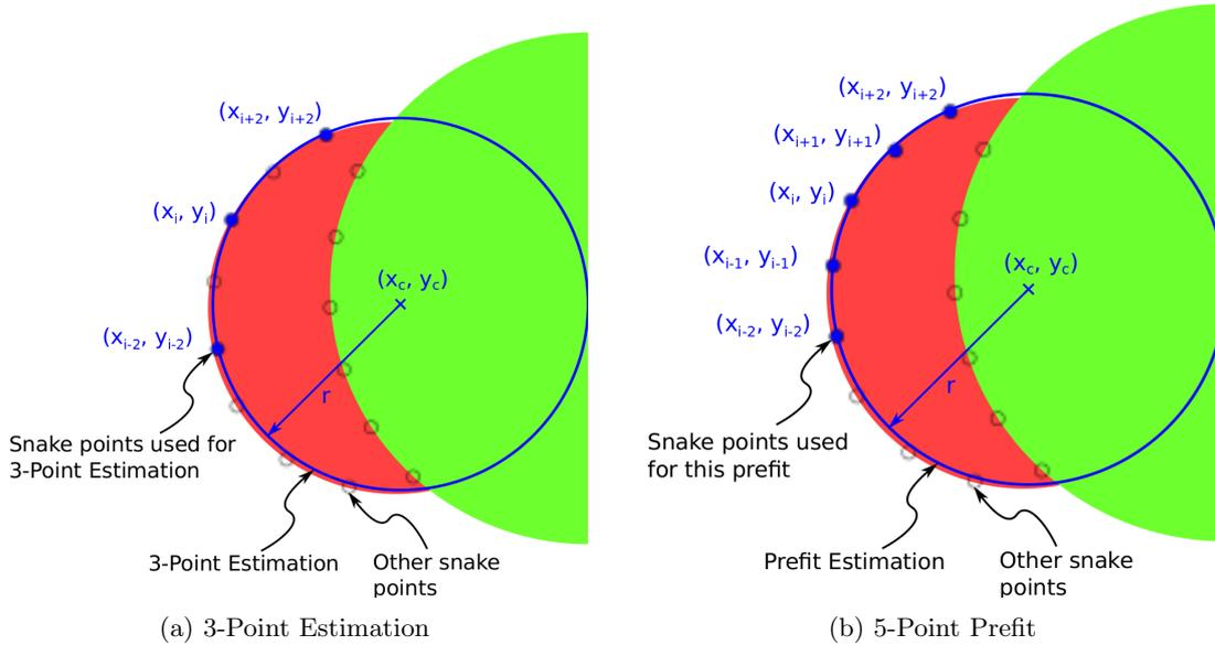
Figure 3.3.: Comparison of the different sets of points used for the estimation around  $i$ -th snake point.
