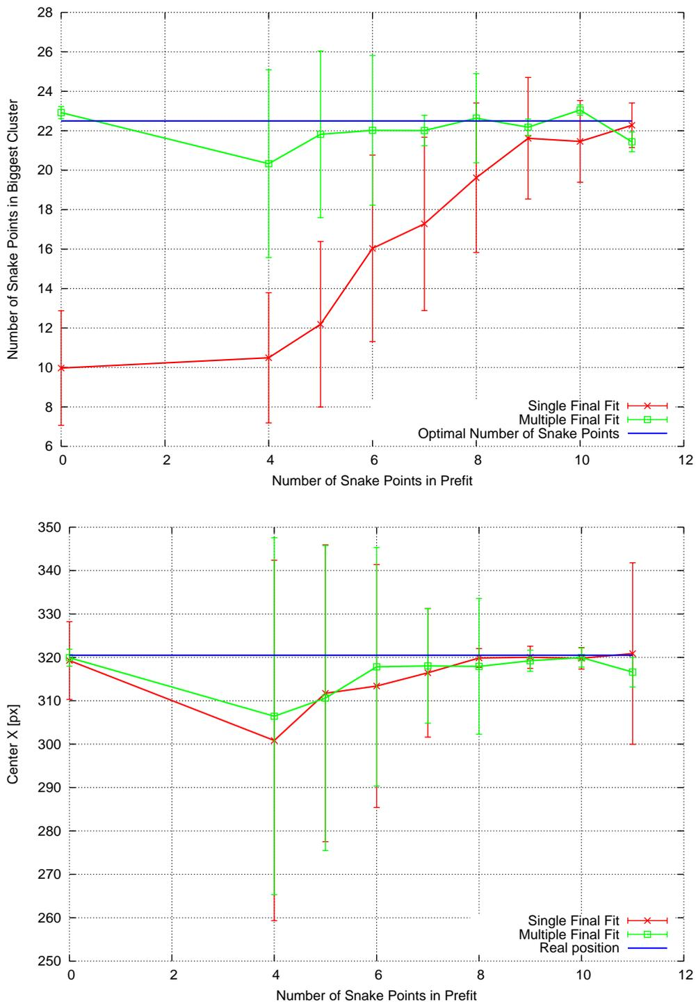
Figure 3.8.: Accuracy of the size of the biggest cluster and  $x_c$  in dependency of the number of prefit points. The result for the three point estimation is given at zero prefit points.
