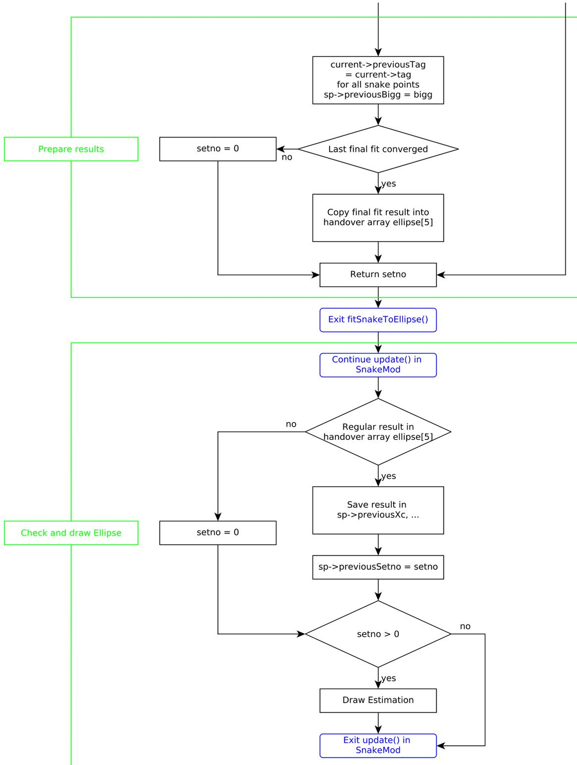
Figure A.4.: Detailed Flowchart of Ellipse Identification Algorithm - Part 4
