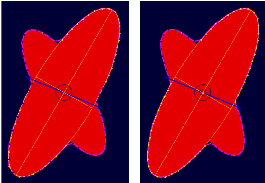
(a) Single Final Fit ignoring data of previous time step. (b) Multiple Final Fit with data of previous time step.
