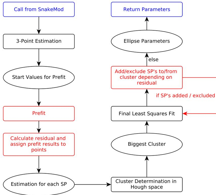
Figure 3.2.: Flowchart of the disk identification algorithm. Red parts are added for this work in order to improve identification.
