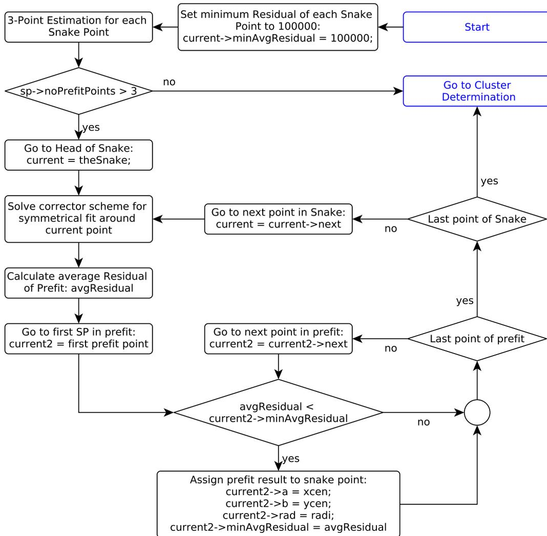
Figure 3.6.: Flowchart of the residual-based assignment of the prefit results.
