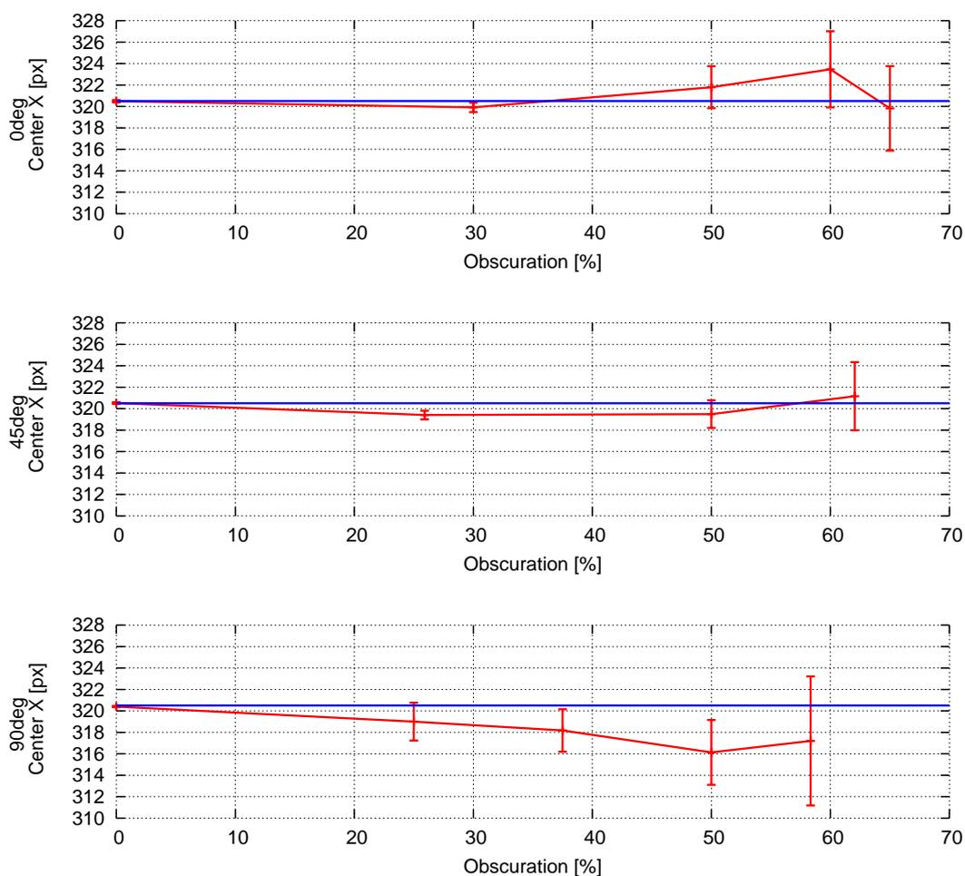
Figure 4.8.: Mean  $\mu_{x_c}$  and standard deviation  $\sigma_{x_c}$  of  $x_c$  depending on grade of obscuration.
