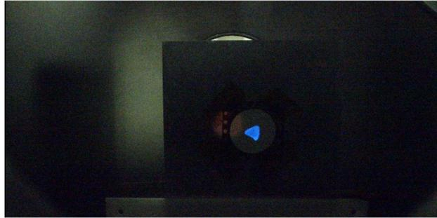
Figure 3.13: Electron beam focused and aligned to center of Ti target plate.
