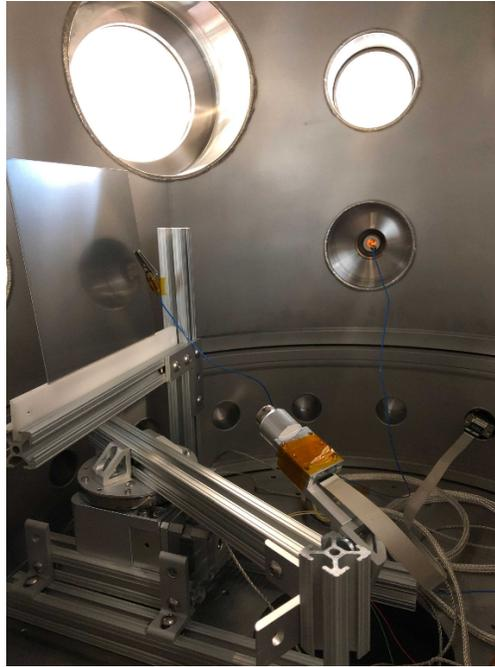
Figure 3.18: Experimental setup for fixed plate, rotating sensor tests.
