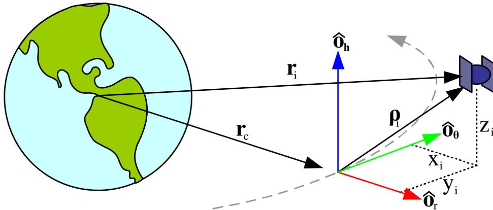
Figure 2.1: Illustration of rotating Hill coordinate frame.
