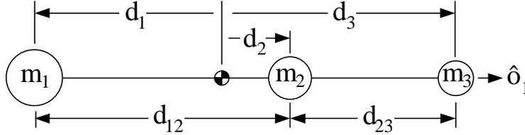
Figure 3.2: Three-spacecraft formation aligned with an arbitrary axis.
