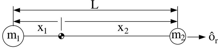
Figure 3.1: Two-spacecraft formation aligned with the  $\hat{o}_r$  axis.
