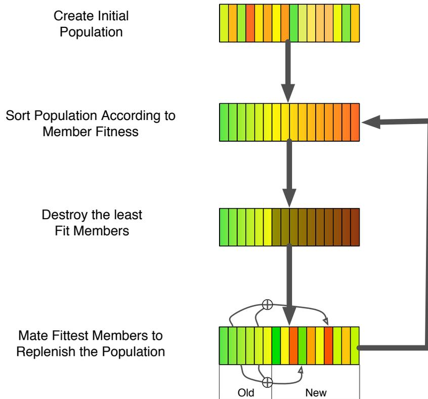
Figure 4.1: Illustration of the single-processor genetic algorithm.
