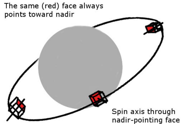
Figure 1.2: Orientation of the CubeSat, where the same face always points toward nadir
