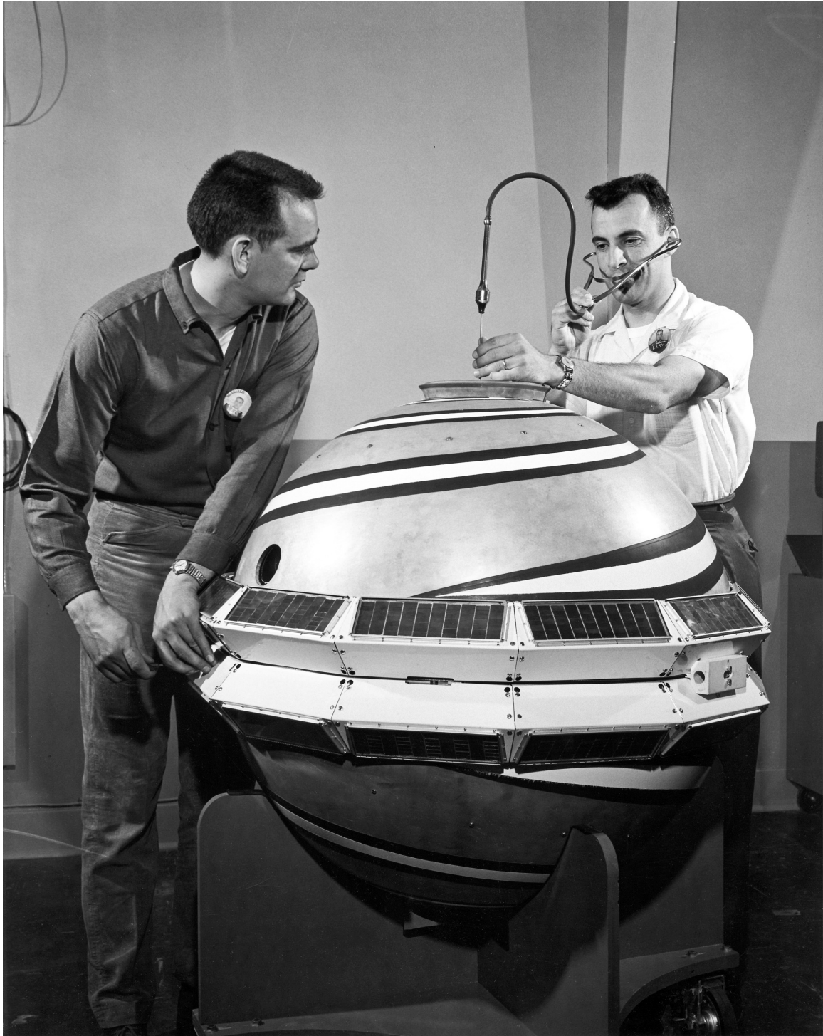
Figure 3.1: The Transit 1B Satellite, the first satellite to use Passive Magnetic Attitude Stabilization. [1]
