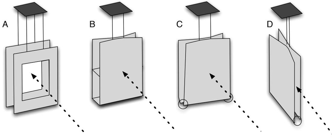
**Figure 13: Four membrane structure configurations A–D used for experiments. The incoming charge flux direction is shown through the dashed arrow.**
