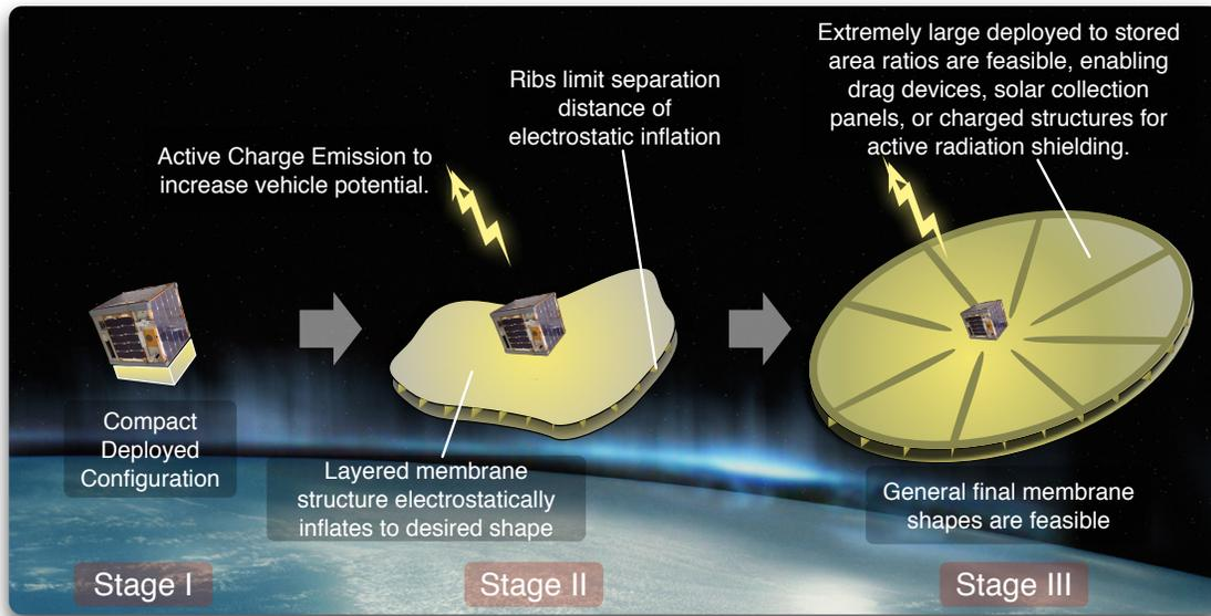
**Figure 1: Electrostatic inflation concept illustration.**
