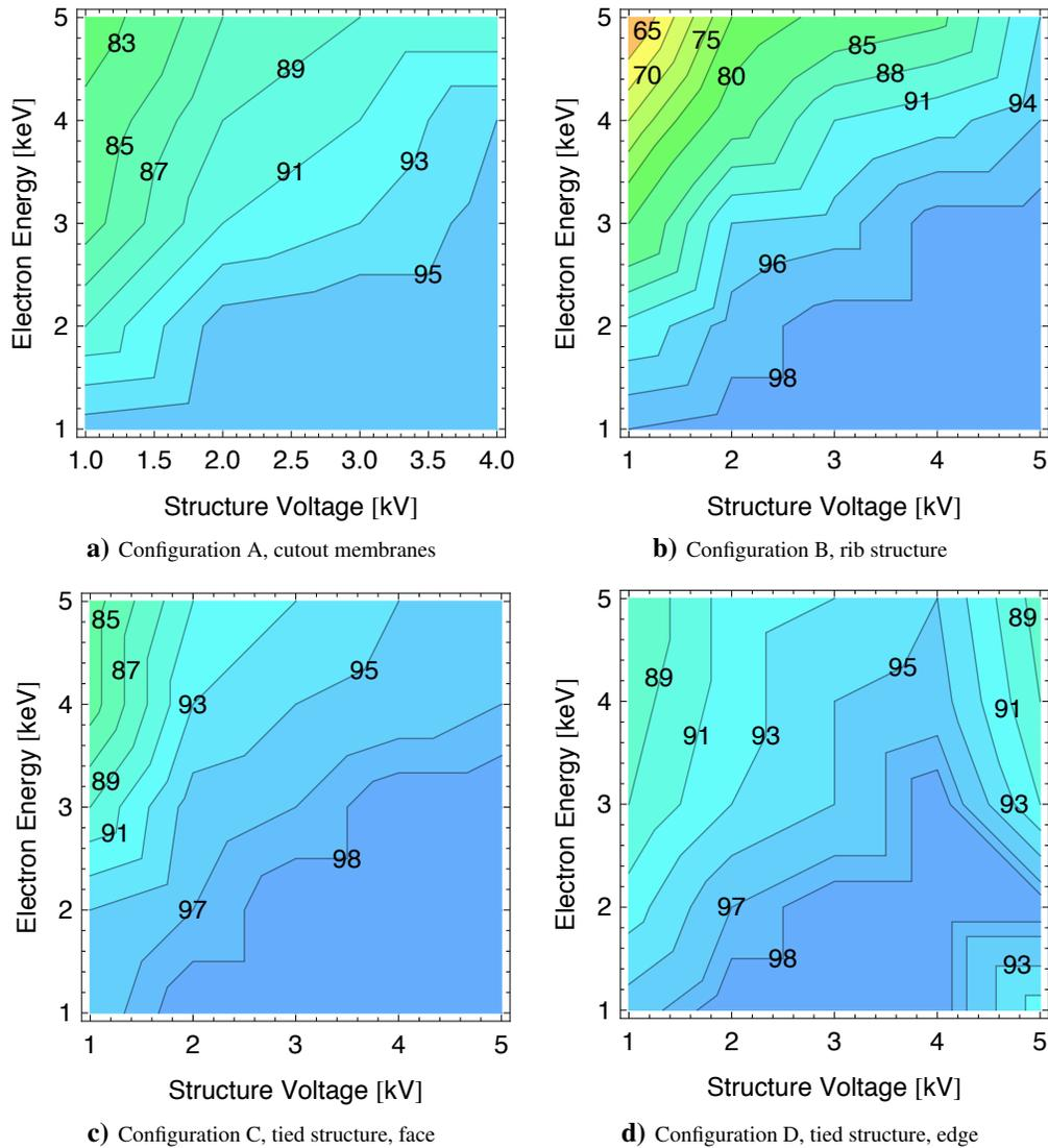
**Figure 14: Percentage of original detected current behind inflated membrane structure at different electron energies**
