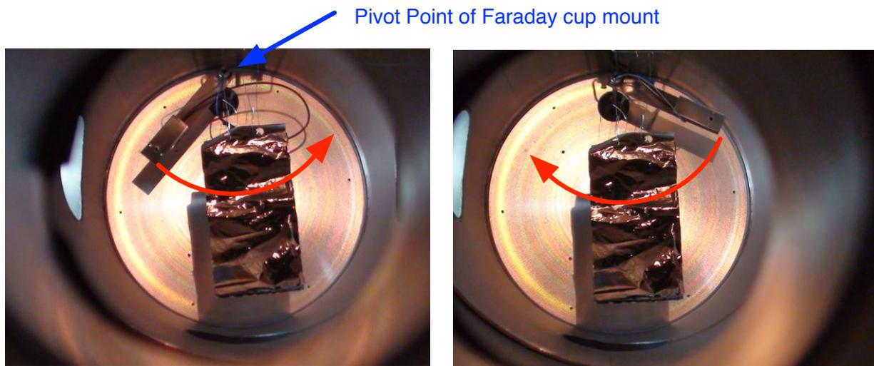
**Figure 11: Rotation of the Faraday cup around the membrane structure**
