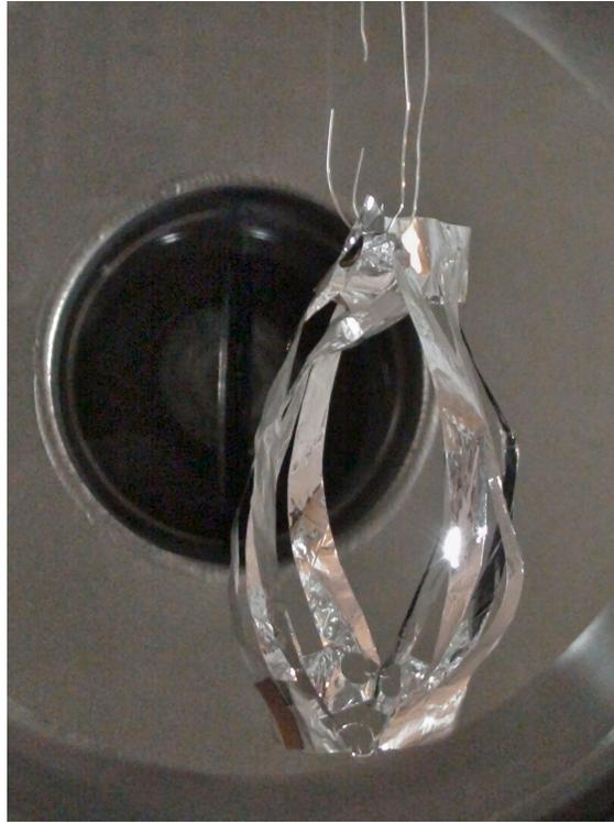
**Figure 6: Inflated structure in vacuum chamber**
