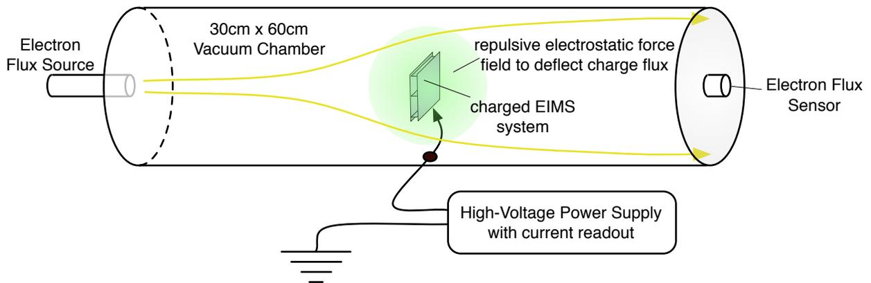
**Figure 7: Concept illustration for the radiation shielding experimental setup**
