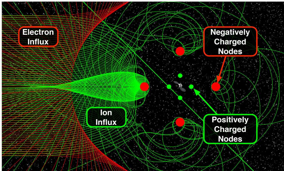
Figure 4: Electrostatic space radiation shielding concept for a deep space application
