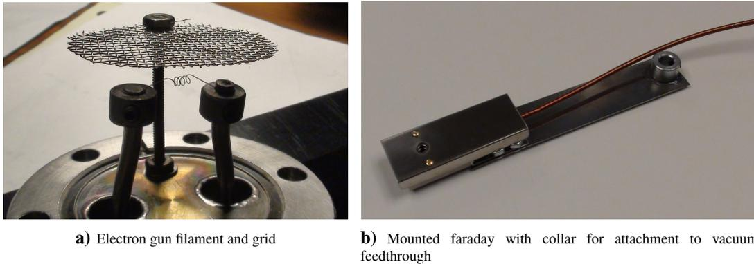
**Figure 9: Charge deflection experiment hardware**
