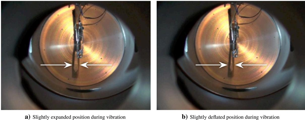
**Figure 10: Video snapshots to illustrate magnitude of structural oscillation; As shown by arrows, difference enhanced in shadow**
