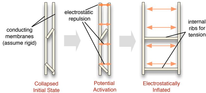
**Figure 2: Sample open-ended membrane rib structure undergoing electrostatic inflation**
