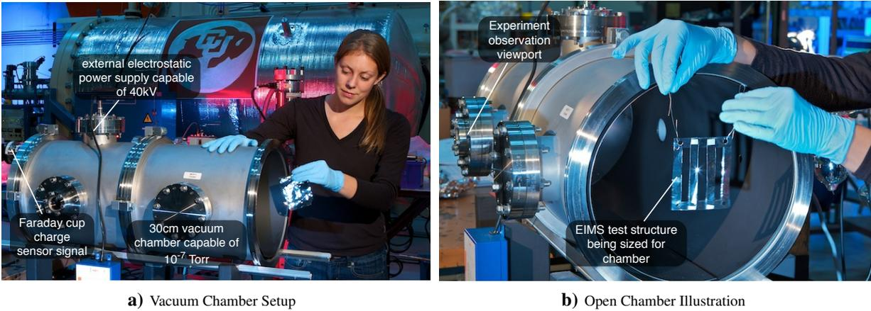
**Figure 8: Charge Flux Experiment Configuration.**
