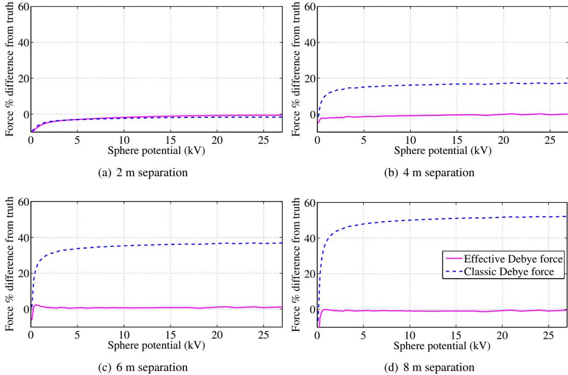
**Figure 10. Comparison of analytic forces with classic and effective Debye lengths as a percentage difference from truth between a 1 m diameter sphere and point charge over a range of CFF potentials for four different separations in a quiet GEO plasma ( $\lambda_D = 4$  m)**
