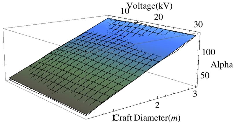
**Figure 7. Alpha parameter values and surface plot of regression (Equation (20)) for LEO plasma conditions,  $\lambda_D = 0.011$ ; colored surface represents data and mesh represents fit surface**
