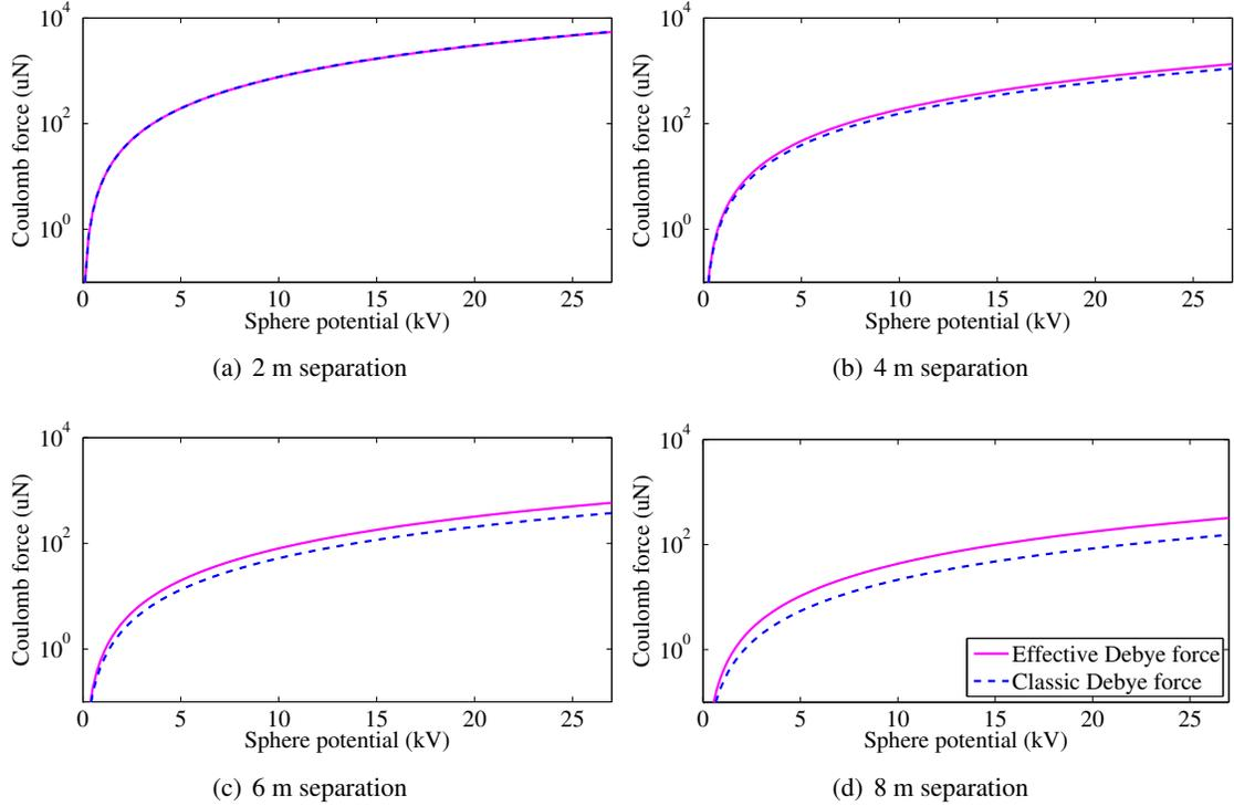
**Figure 9. Force between a 1 m diameter sphere and point charge over a range of CFF potentials for four different separations in a quiet GEO plasma ( $\lambda_D = 4$  m)**
