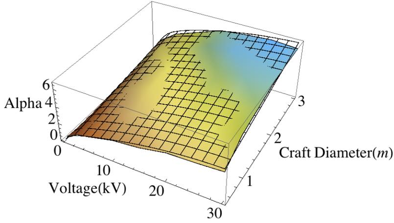
**Figure 5. Alpha parameter values and surface plot of regression (Equation (19)) for Quiet GEO plasma conditions,  $\lambda_D = 4$ ; colored surface represents data and mesh represents fit surface**
