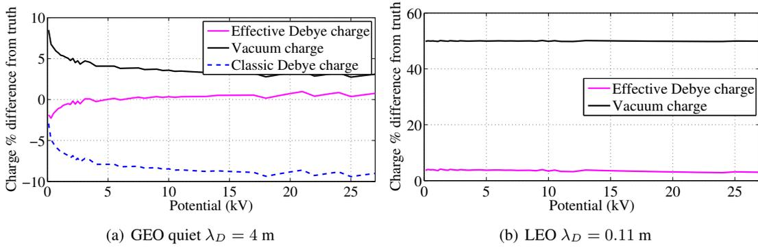
**Figure 8. Computation of charge on an isolated sphere using analytic models compared to the numerical truth as a percentage difference over a range of CFF potentials**
