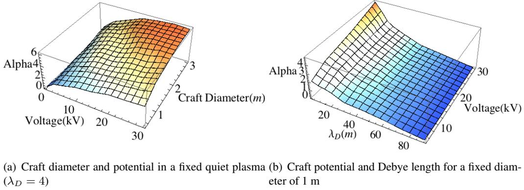
**Figure 3. Trends in Alpha parameter for effective Debye lengths in a GEO plasma**
