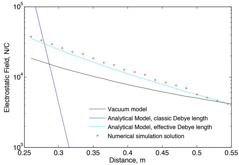
**Figure 6. Comparison of classic E-field models with the effective Debye model; LEO plasma,  $\lambda_D = 0.011m$ ,  $V_C = 5kV$**
