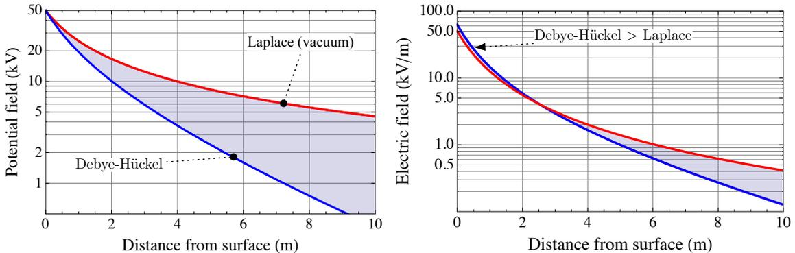
**Figure 2. Potential and electric fields from an isolated, 1 m sphere diameter charged to 50 kV (quiet GEO plasma,  $\lambda_D = 4$  m, used for the Debye-Hückel model)**
