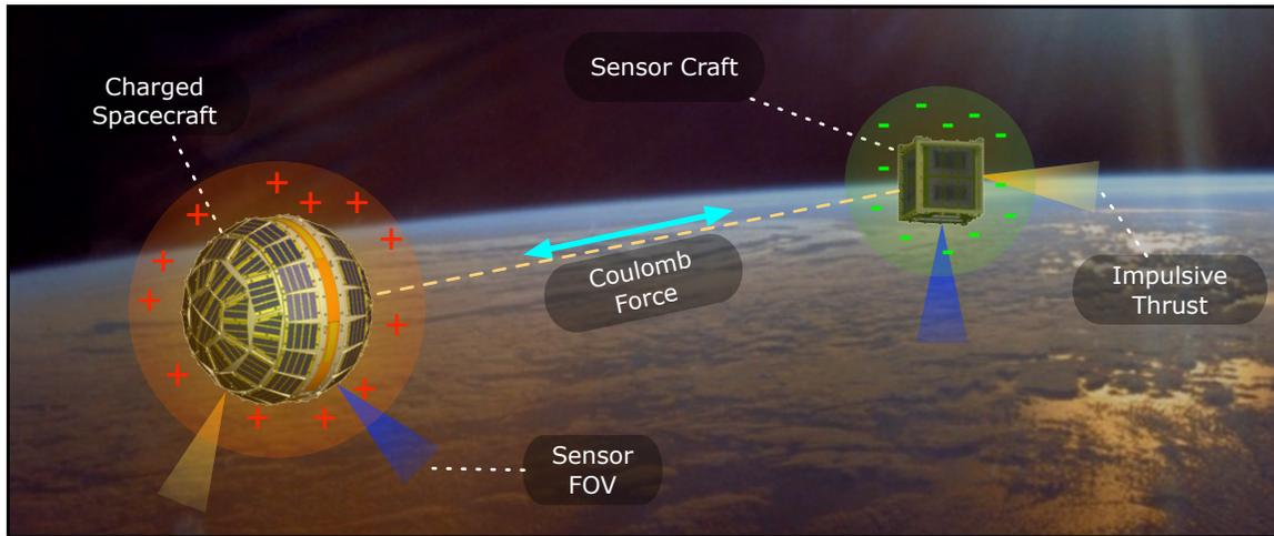
**Figure 1. Two-craft Coulomb formation flight concept; active charge emission is used to charge craft to kilovolt-level potentials to control the separation distance with electrostatic forces**
