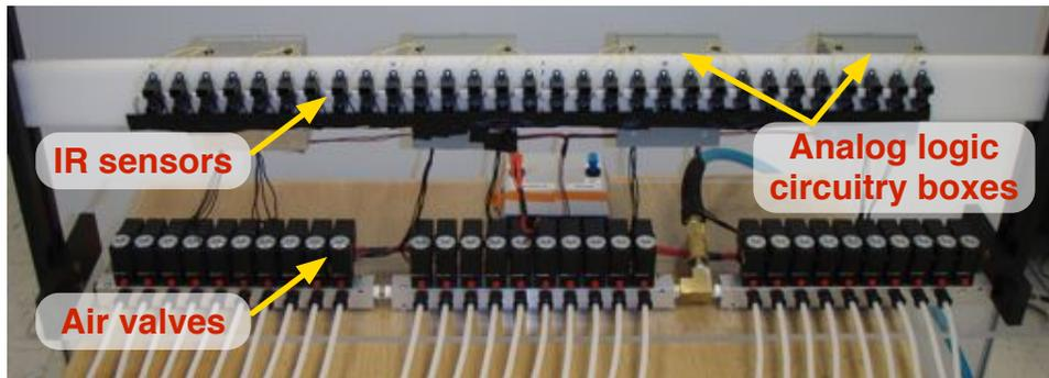
**Figure 5. Autonomous air flow control system with IR sensors and air valves**
