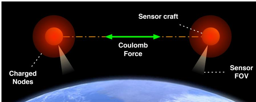
**Figure 1 Two sensor nodes using Coulomb forces to provide the necessary formation separation distance.**
