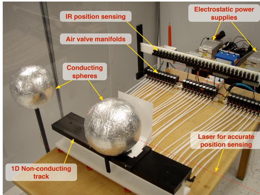
**Figure 3. Model of laboratory Coulomb testbed**
