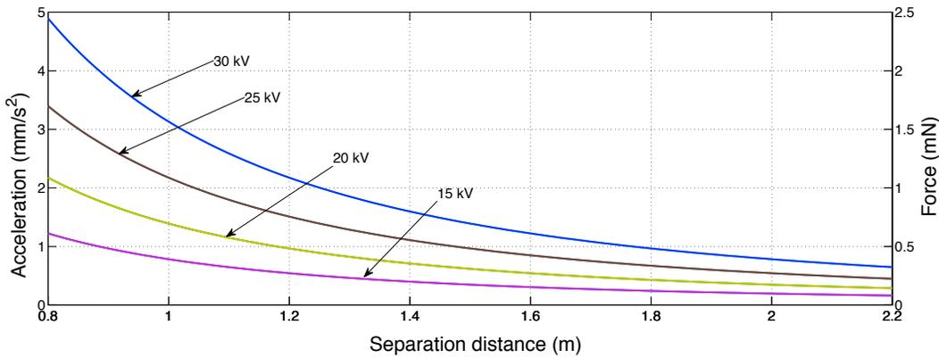
**Figure 2 Anticipated Coulomb force and vehicle acceleration for a 0.5 kg cart, spheres of diameter 25 cm voltages of 15-30 kV.**
