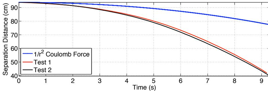
**Figure 10 Coulomb attraction tests conducted with a cart initially at rest and attracted with cart at +30 kV and stationary sphere at -30 kV**
