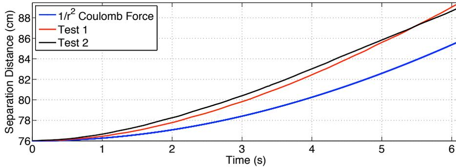
**Figure 9 Coulomb acceleration tests conducted with a cart initially at rest and re-pulsed with +30 kV potentials on both spheres**
