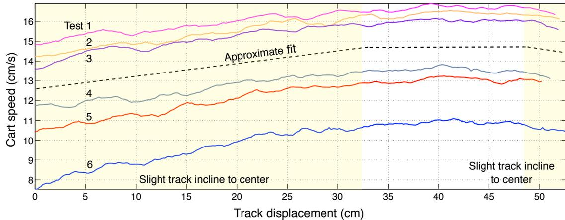
Figure 8. Cart speed as function of track distance (low pass filtered)
