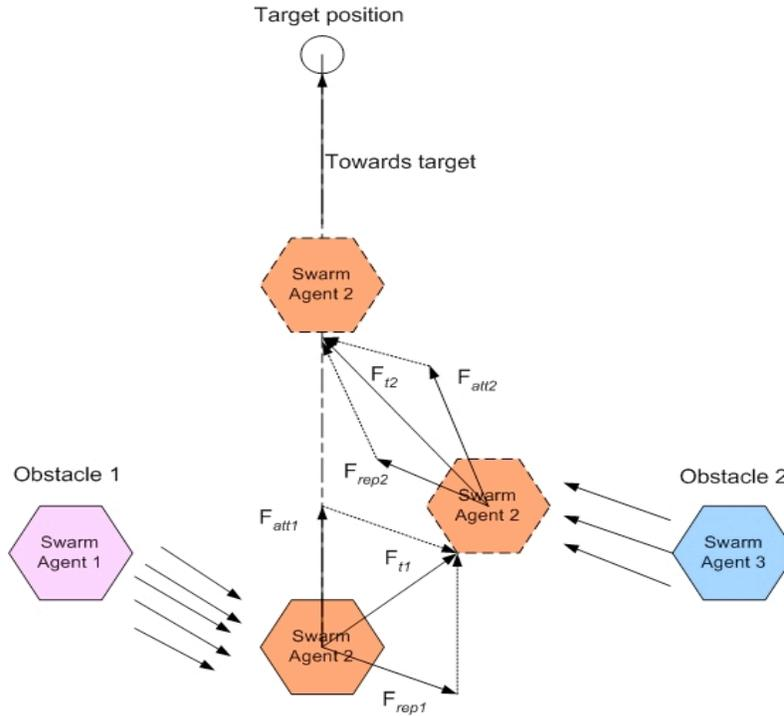
**Figure 1. Schematic diagram of path planning using APF method**
