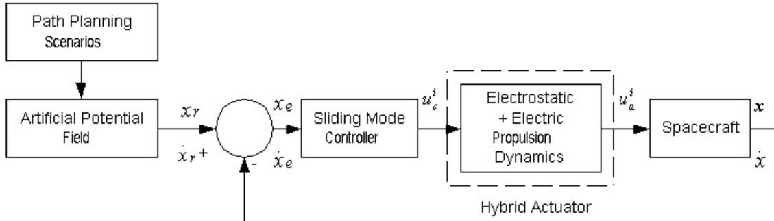
**Figure 2. Schematic diagram of swarm path planning and control with hybrid actuator**
