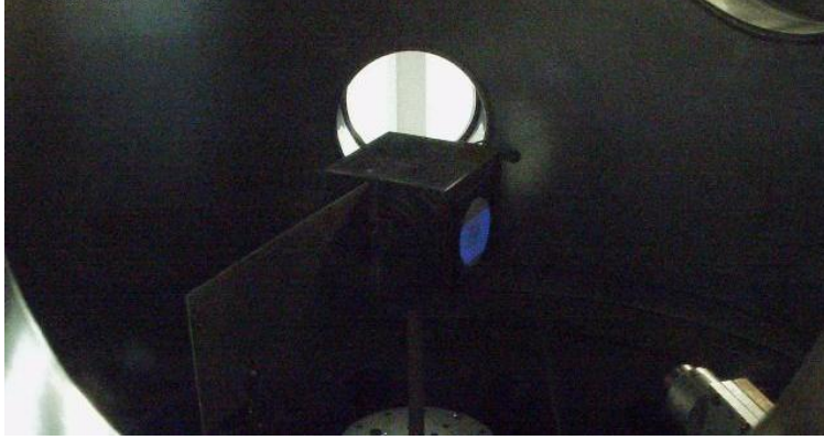
Fig. 9 Wide Electron Beam for measuring multiple potentials simultaneously
