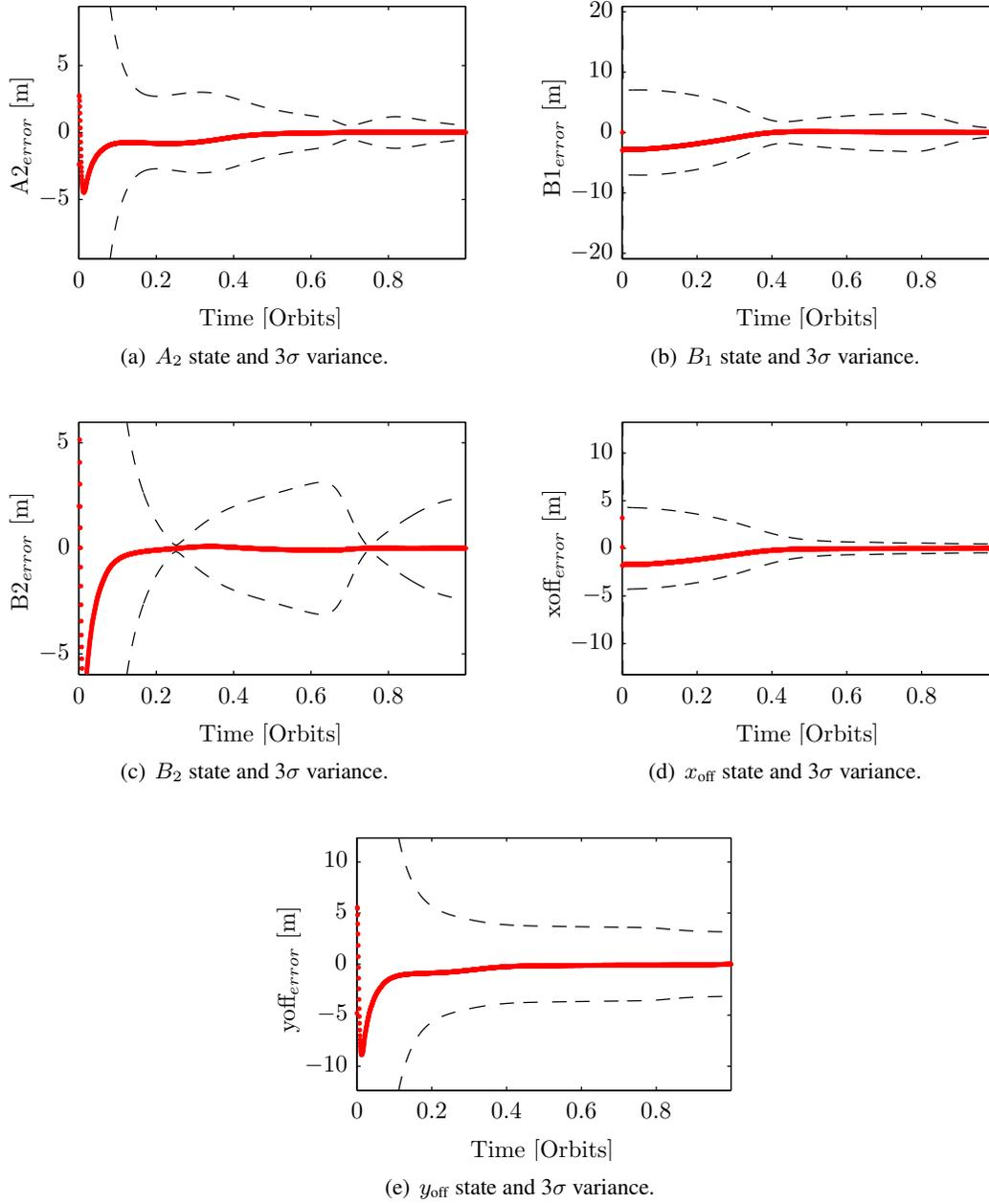
**Figure 4. LROE estimated state error and covariance envelopes demonstrating the boundedness of the along-track offset relative ellipse estimate with large initial error.**
