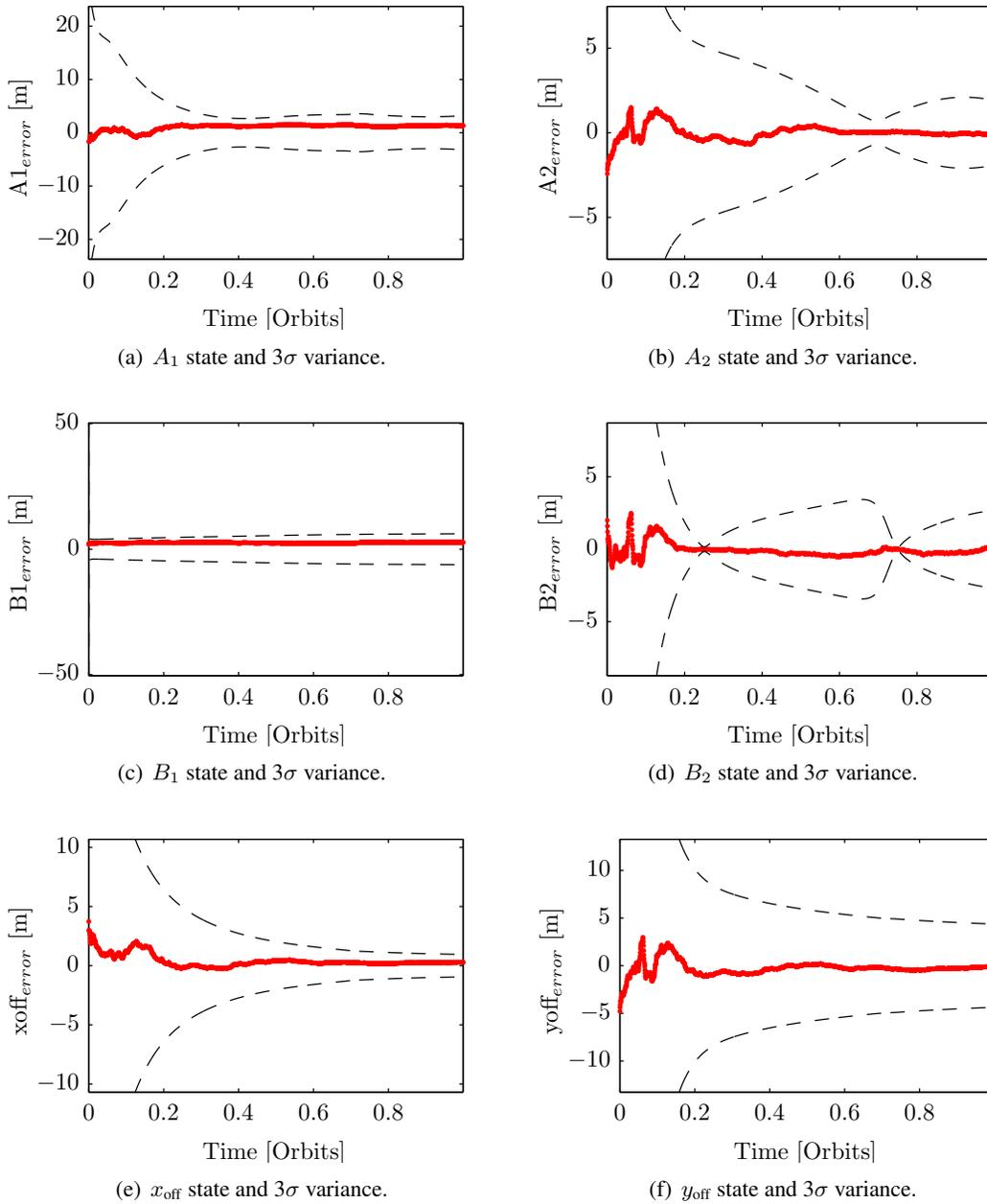
**Figure 3. LROE estimated state error and covariance envelopes demonstrating the converging trend of the drifting relative ellipse estimate.**
