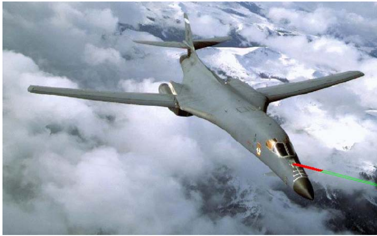
Figure 11. Exaggerated Illustration of the Shape of the Range (Red) and Heading Errors (Green) from air Refueling Visual Position Sensing Simulation.
