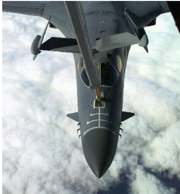
Figure 1. B-1B Lancer Refueling From a KC-10 Extender Using the Boom and Receptacle Method
