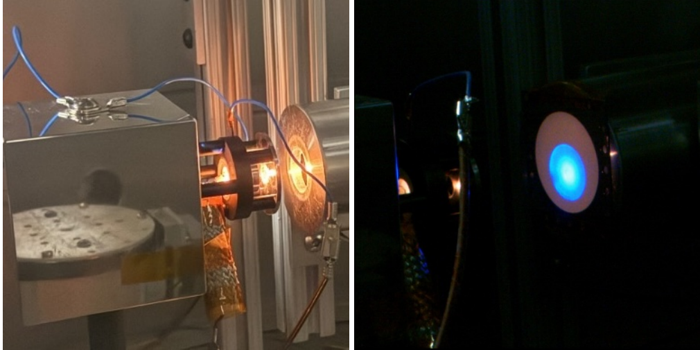
(a) Floating electron-gun spacecraft analog installed in the ECLIPS vacuum chamber. (b) Electron beam intercepted by the phosphor screen during source characterization.
