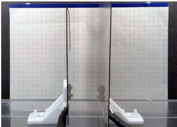
(b) Plate and Wire Charged to 3kV
