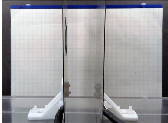
**Figure 1.37:** 28AWG Wire Charged to 17.2kV and Exposed to  $389\frac{kV}{m}$  Electric Field
